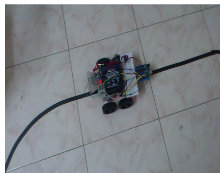
Fig.4 Shows the robot following the line
