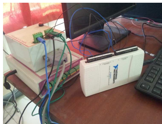
Figure 2: Interfaced NI-Daqmx 6211 Data Acquisition Module Card.
