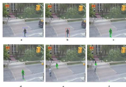
Fig. 5 (a). Original frame, (b) Manually selected object (man) to be tracked, (c), (d), (e) Object tracked in subsequent frames using KLT algorithm.
