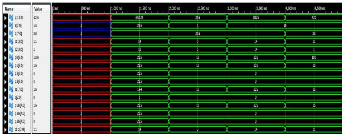
Figure 11: Simulation results of Pipelined Vedic Multiplier
