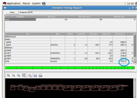
Figure 16: Delay Of Wallace Tree Multiplier
