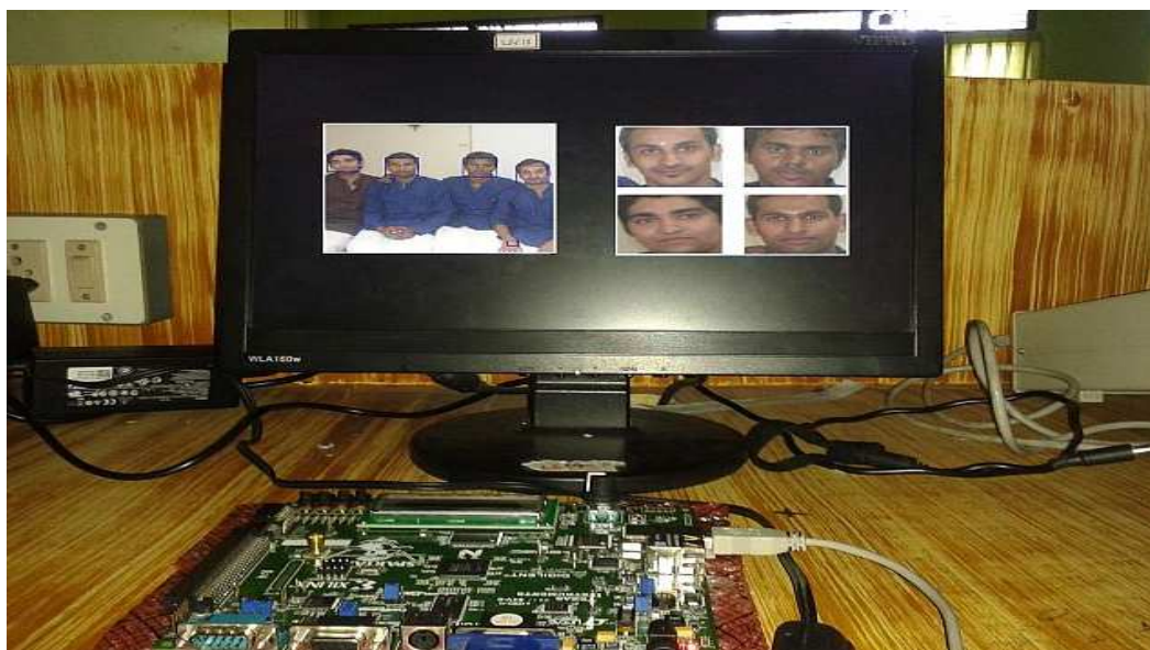
Figure 10: Real Setup using FPGA for Face Detection
