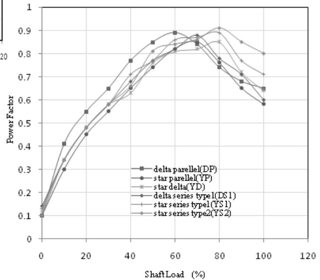
Fig. 18. Power factor as a function of load for DP, YP, YD, DS1, YS1 and YS2 optimum design connections.
