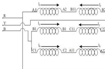
Fig. 13. Delta-series type III (DS3) Connection.
