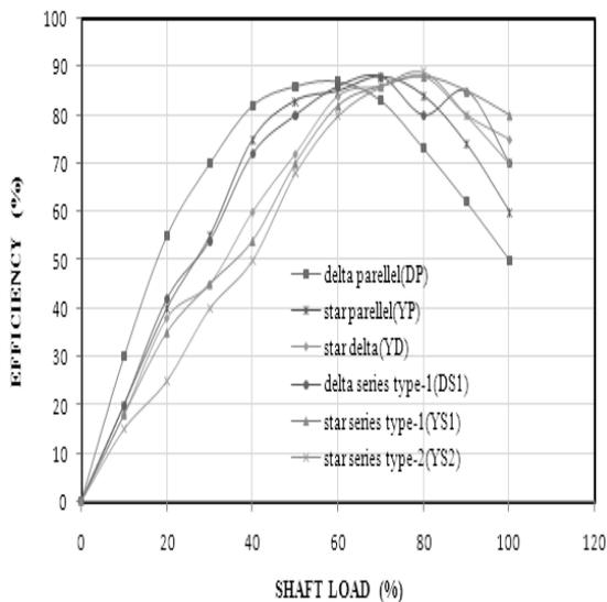
Fig. 15. Efficiency as a function of load for DP, YP, YD, DS1, YS1 and YS2 conventional design connections .
