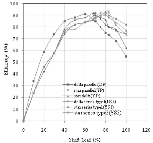
Fig. 17. Efficiency as a function of load for DP, YP, YD, DS1, YS1 and YS2 optimum design connections.
