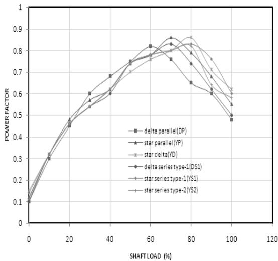
Fig. 16. Power factor as a function of load for DP, YP, YD, DS1, YS1 and YS2 conventional design connections
