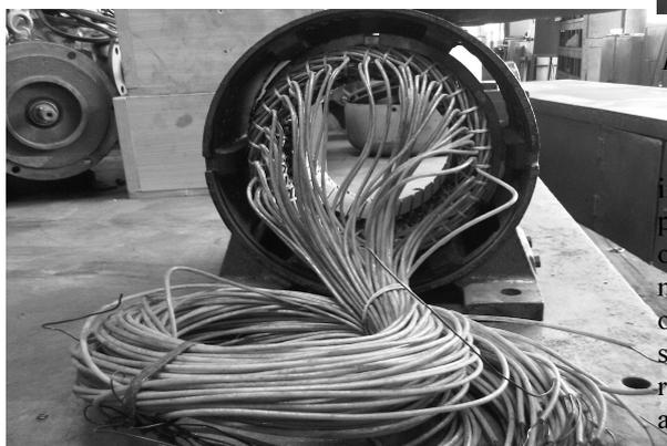
Fig. 19. 2.2- kW Multi-flux Stator winding for different connections
