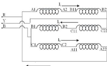
Fig.11. Delta-series type II (DS2) Connection.
