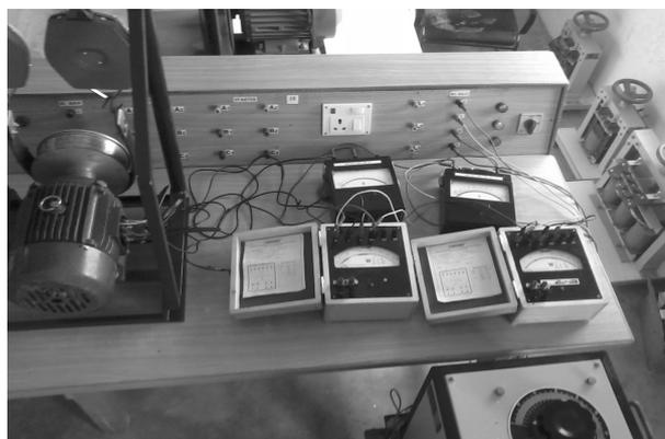
Fig. 21. Experimental setup for 2.2- kW multi-flux stator double layer winding SCIM
