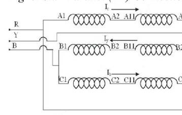
Fig. 7. Delta-series type I (DS1) Connection.
