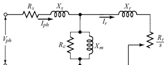
Fig. 1. Equivalent circuit of three phase SCIM.
