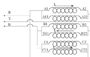
Fig. 5. Delta Parallel (DP) Connection.
