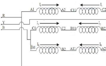
Fig. 14. Delta-series type IV (DS4) Connection.
