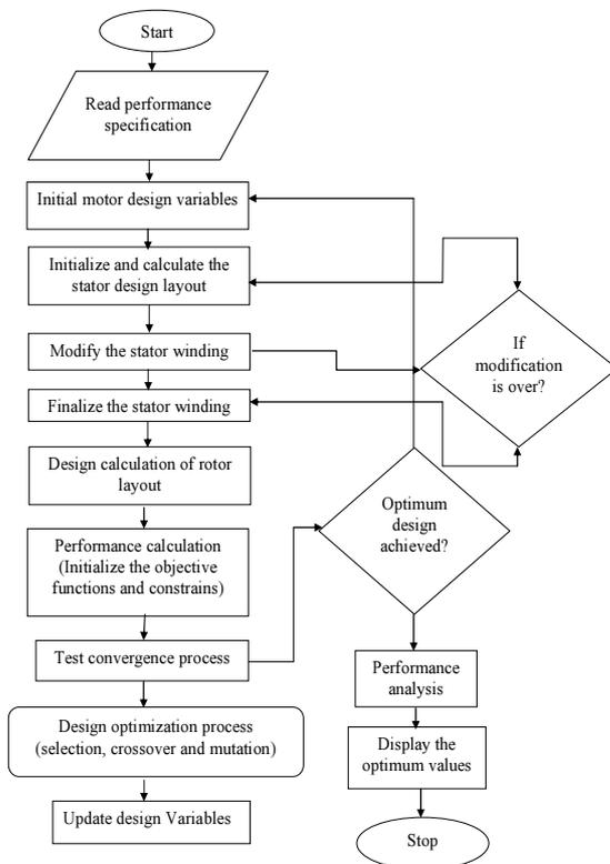
Fig. 3. Flow chart for design and GA-based optimization process.
