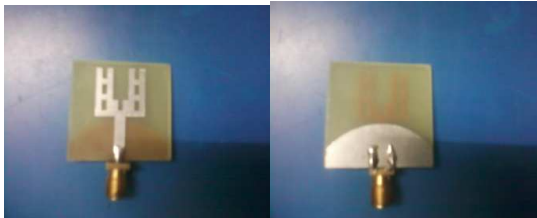
Figure 5: Fabricated Second Order Fractal Antenna With Half Arc Ground Plane
