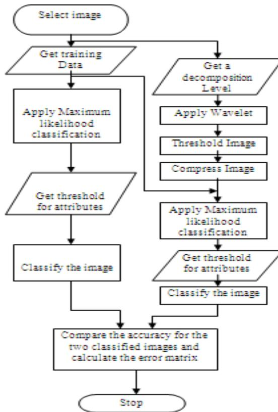
Figure 10 : Flow Chart Of The Above Technique
