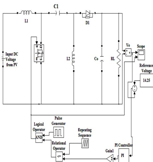
Fig 7. SEPIC Simulation Implemented In MATLAB
