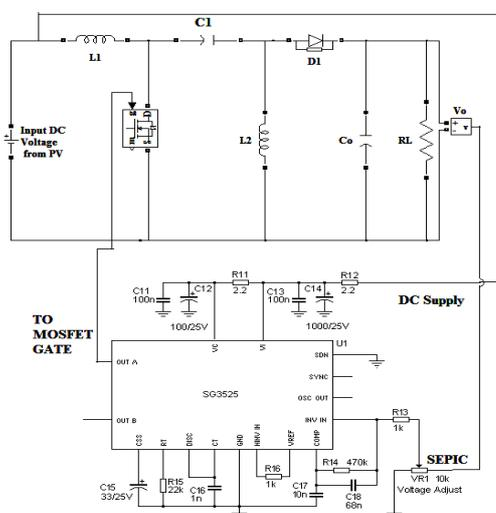
Fig. 15 Sepic With Pulse Width Control Circuit Sg3525
