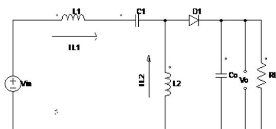
Fig .5 SEPIC current flow when S1 is in OFF condition.
