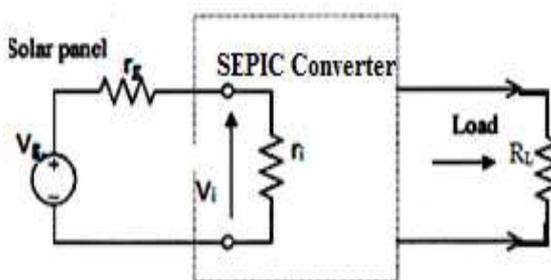
Fig.1 Equivalent Circuit Of PV With Converter.
