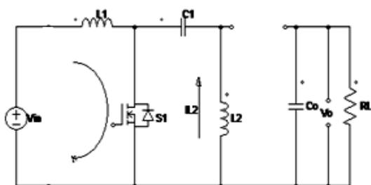
Fig.4. SEPIC current flow when S1 is in ON condition.
