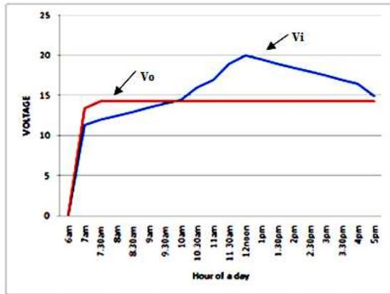
Fig.16. Plot Of  $V_i$  And  $V_o$  Variations During A Day
