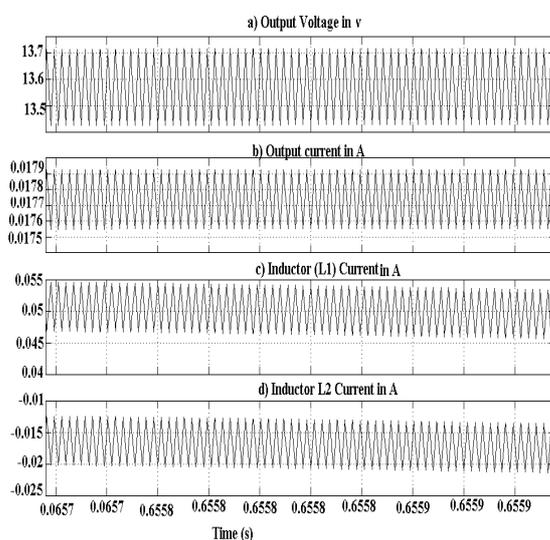
Fig.11.Simulated A) Output Voltage And B) Output Current Waveforms, Of SEPIC C) Inductor(L1) Current And D) Inductor (L2)Current.
