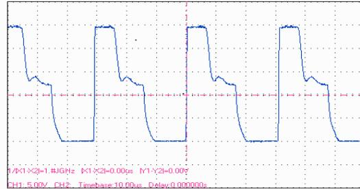
Fig.19. Output Voltage Waveform At 11.3V DC Input
