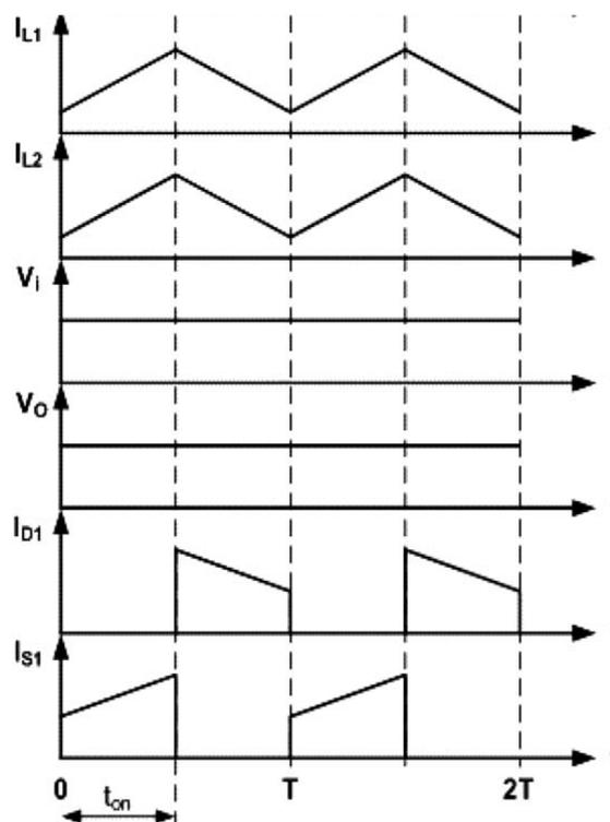
Fig.6.Theoretical WAVEFORM OF Sepic CONVERTER
