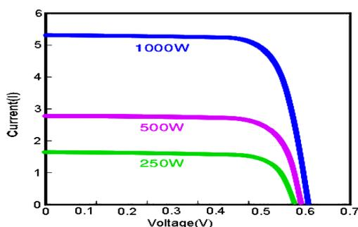
Fig. 2 PV Panel I-V Characteristics
