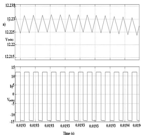
Fig.9 Simulated Output Voltage Waveform Across C1 and L1
