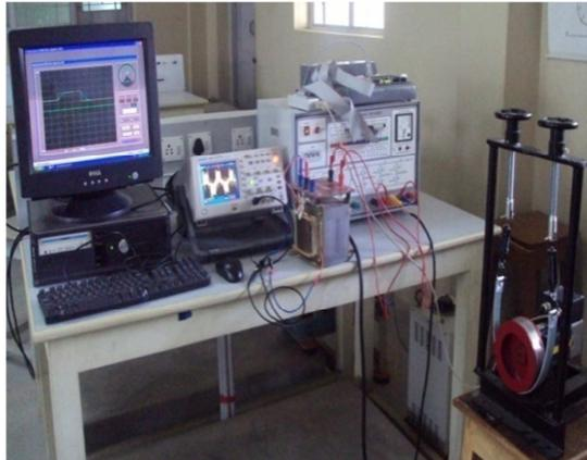
Fig.11. Experimental Setup using TMS320F2812 Processor
