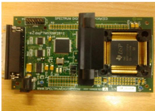
Fig.12. TMS320F2812 DSP board
