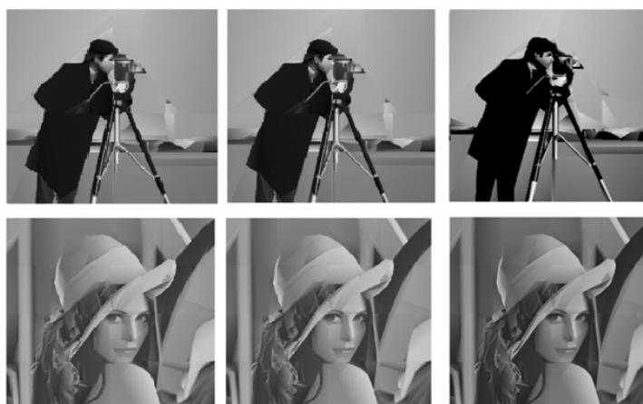
Figure 7. Top Left: Reconstructed Cameraman using the normal form of straight line in GW Algorithm, 0.0625 bpp, PSNR=22.93. Top Center: Reconstructed Cameraman using the slope-intercept form of straight line in GW Algorithm, 0.0625 bpp, PSNR=23.04. Top Right: Reconstructed Cameraman using the Proposed Method, 0.0625 bpp, PSNR=24.55. Bottom Left: Reconstructed Lena using the normal form of straight line in GW algorithm, 0.0625 bpp, PSNR=28.72. Bottom Center: Reconstructed Lena using the slope-intercept form of straight line in GW Algorithm, 0.0625 bpp, PSNR=28.78. Bottom Right: Reconstructed Lena using the Proposed Method, 0.0625 bpp, PSNR=29.73.
