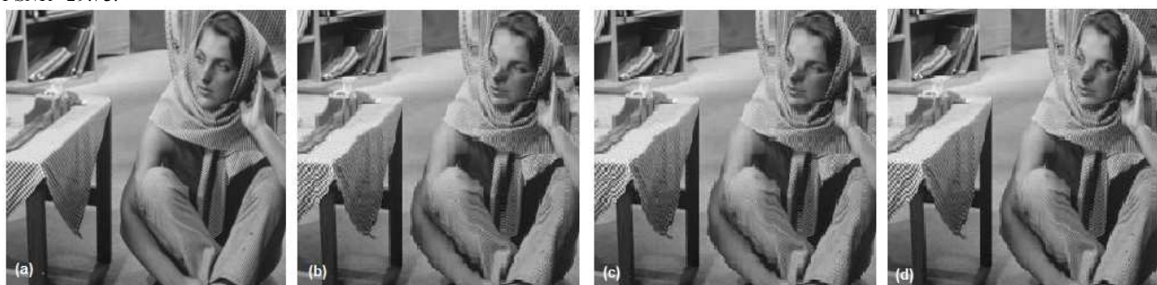
Figure 8. (a): Original Barbara (512x512). (b): Reconstructed Barbara using the normal form of straight line in GW Algorithm, 0.0625 bpp, PSNR=26.04. (c): Reconstructed Barbara using the slope-intercept form of straight line in GW Algorithm, 0.0625 bpp, PSNR=26.45. (d) Reconstructed Barbara using the Proposed Method, 0.0625 bpp, PSNR=27.32.
