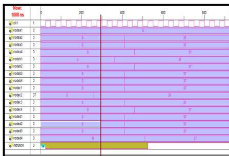
Figure 10: Node-Level Detection In The Absence Of A Ship's Intrusion
