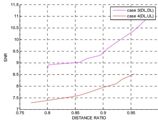
Fig. 10. SNR vs. distance ratio Case3 and Case4
