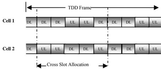
Fig.2. Different slot allocation in a adjacent cell
