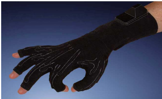
Figure 3: The 5DT Data Glove Ultra 14
