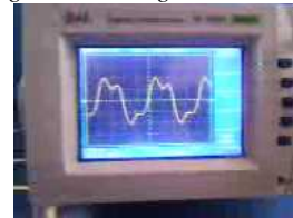
Figure 5. Line to ground fault In Figure 5 the Line to ground fault and the signal pattern is captured. The Figure 6 shows the Measuring probe and Flux sensor which used for the signal pattern collections.
