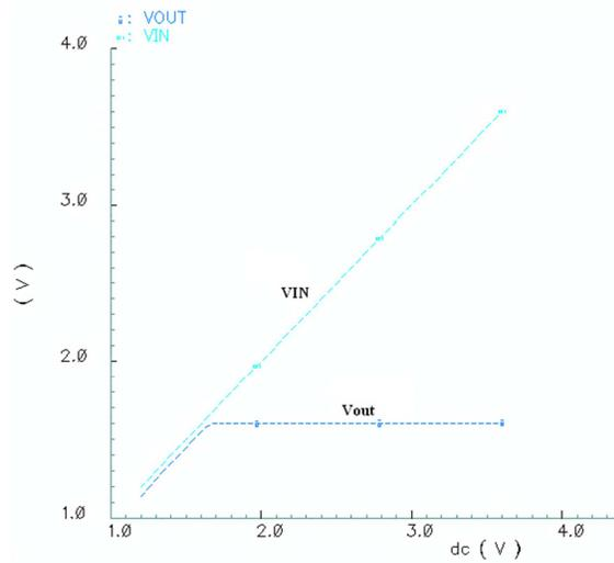
Figure 6: DC line regulation simulation.
