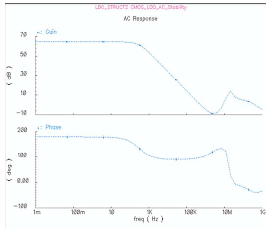
Figure 3: Simulation Result Of Proposed LDO Frequency Response.
