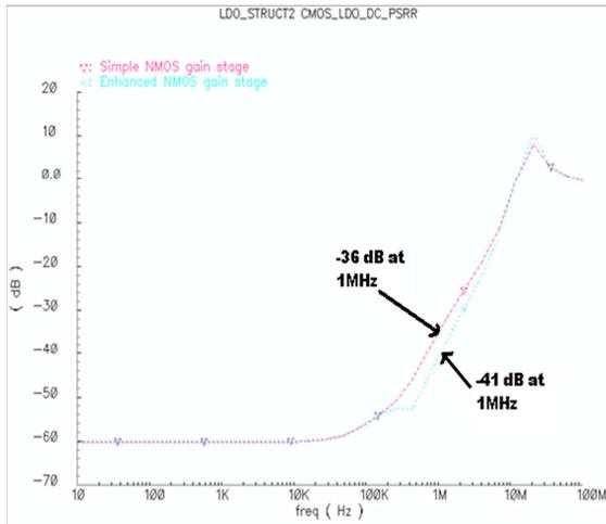
Figure 4: PSRR simulation performance of the proposed full on-chip LDO.
