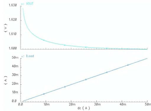
Figure 7: DC line regulation simulation.
