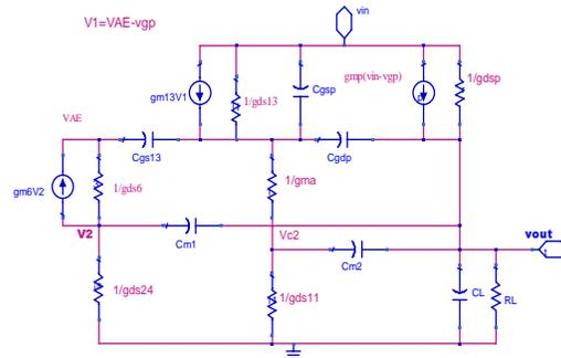
Figure 2: Small signal model of enhanced PSRR.
