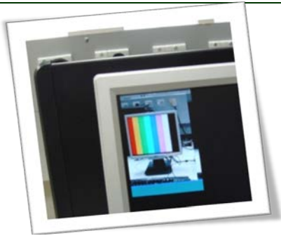
Color Image 1 Displayed With VGA Controller Snap Shot .
