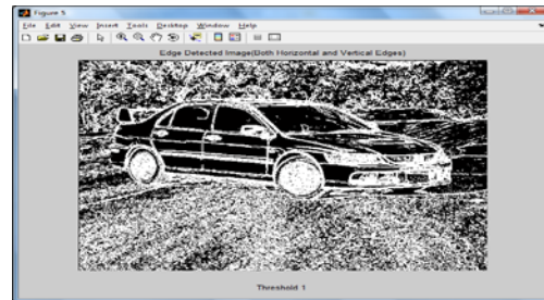
Both Horizontal And Vertical Edges Detected Image For Threshold 1
