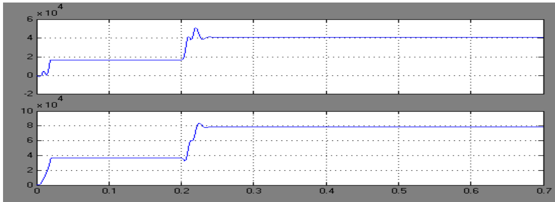
Fig. 3(b). Real And Reactive Power Across Bus-7
