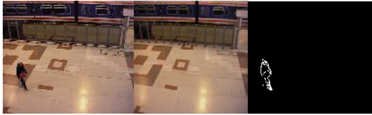
Figure 2. On The Left, The Original Frame, In The Middle, The Background And In The Right Extracted Foreground
