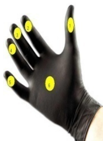
Figure 5: Braille positions in the Glove
