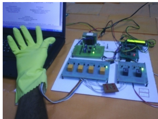
Figure 6: Hardware prototype of Braille hand glove
