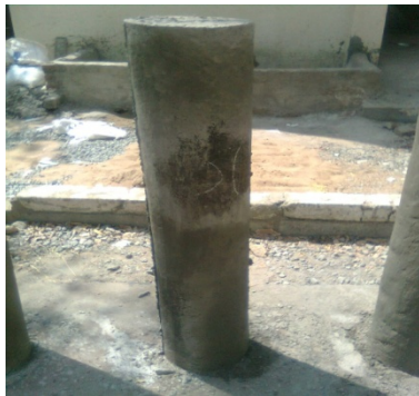
Figure .5c: After Retrofitting Specimen
