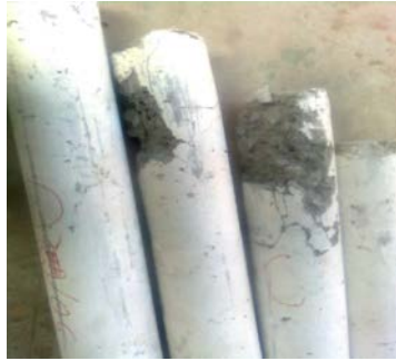
Figure.5a: Before Retrofitting Of Specimen
