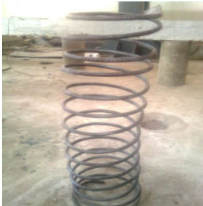
Figure.3: Reinforcement Details Of The Specimen
