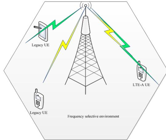
Figure 2: Schematic Presentation Of Frequency Selective Environment With Links Indicating Different Carrier Coverage.
