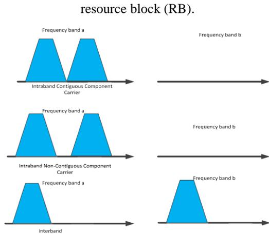
Figure 1: Different Types Of Carrier Aggregation
