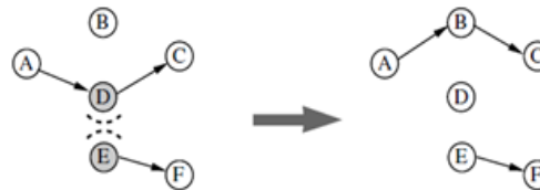
Fig:4 An Example Of Inter Flow Interference
