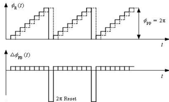
Figure 3. Schematic Diagram Of Ladder Wave Modulation.
