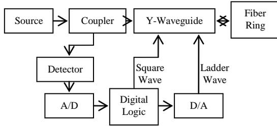
Figure 1. The Frame Of Closed Loop Control System Of FOG.
