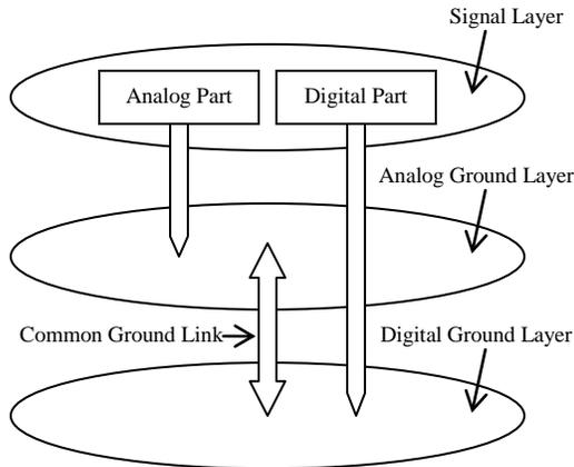
Figure 9. Layout Of Ground For PCB.
