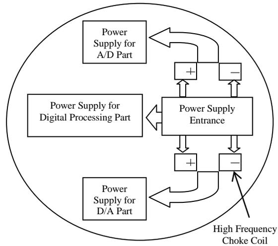
Figure 8. Layout Of Power Supply For PCB.
