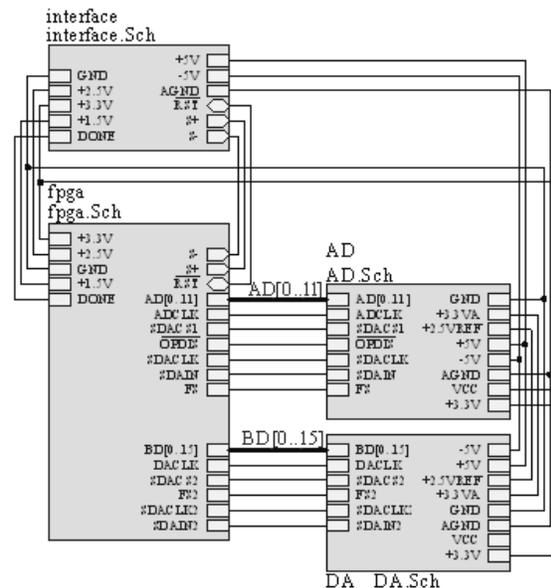
Figure 6. The Connection Diagram Of FPGA.
