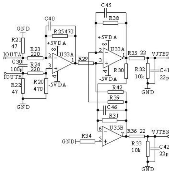
Figure 7. The Circuit Of Post Amplifier.
