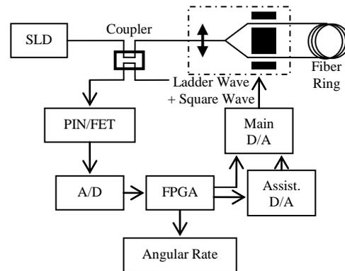
Figure 4. The Frame Of Closed Loop Control System Of FOG Based On FPGA
