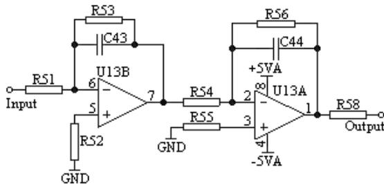
Figure 5. The Circuit Of Preamplifier.
