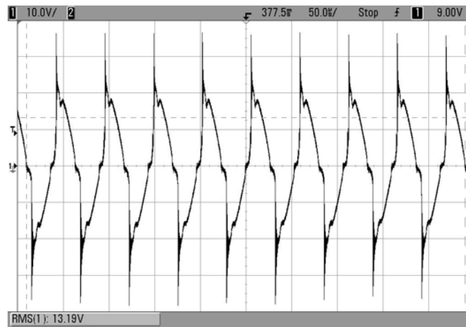
Figure 5 The output voltage waveform of transformer
