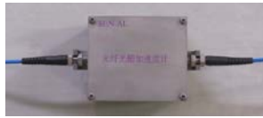
Figure 11. SEN-AL fiber accelerometers.
