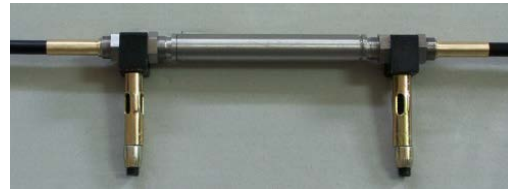
Figure 8. SEN-S1 fiber surface strain sensor.
