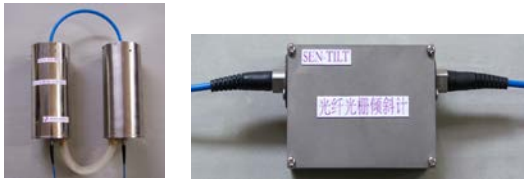
Figure 4. Static level meter. Figure 5. Inclinometers.
