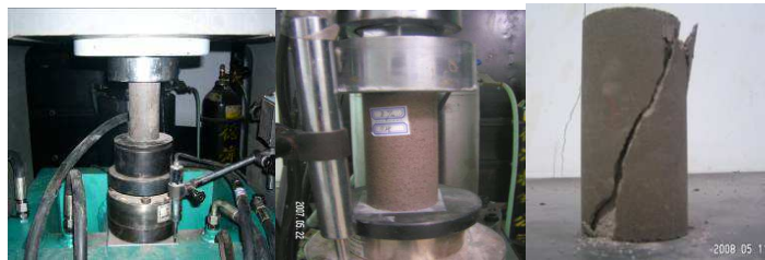
(A) Compressive Strength Test
