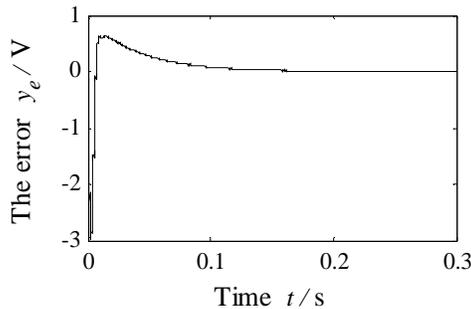
Figure 6. The Error Waveform of Output Voltage for the Boost Converter
