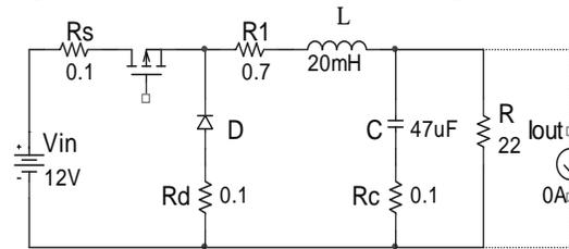
Figure 1. Topology of Buck Converter
