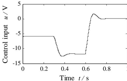
Figure 4. Control Input Response of Buck Converter for Input Voltage Variations
