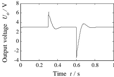
Figure 3. Output Voltage Response of Buck Converter for Input Voltage Variations
