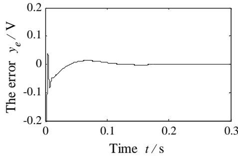
Figure 2. The Error Waveform of Output Voltage for the Buck Converter
