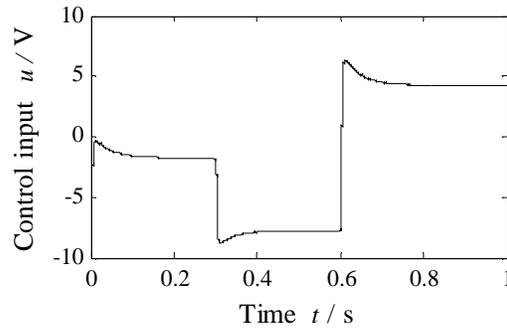
Figure 8. Control Input Response of Boost Converter for Input Voltage Variations
