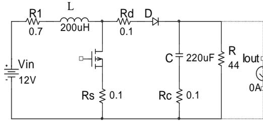
Figure 5. Topology of Boost Converter
