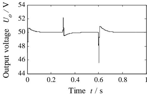
Figure 7. Output Voltage Response of Boost Converter for Input Voltage Variations
