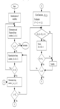
Fig 3:. Flowchart Of Bacterial Foraging Algorithm
