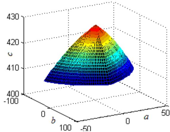
Figure 4: Position-Workspace under the Constraints of Second Group
