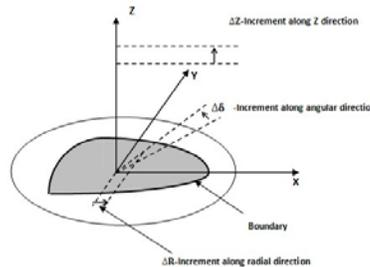
Figure 2: Workspace Limit Boundary Searching Diagram
