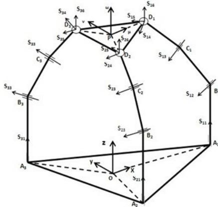
Figure 1: Schematic Representation of a 3/3-RRRS Parallel Manipulator
