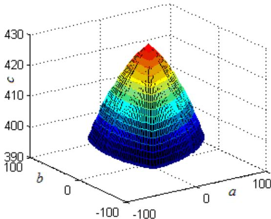
Figure 3: Position-Workspace under the Constraints of First Group
