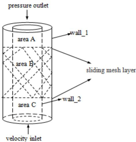
Figure 2: The Boundary Condition Setup
