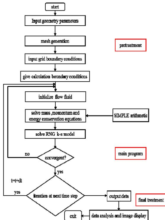
Figure 3: The Program Flow Of The Numerical Calculation
