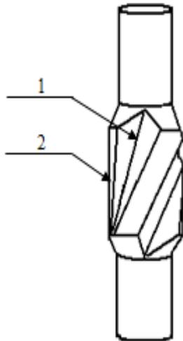
Figure 1: Structure Of The Spiral Centralizer (1-Spiral Flow, 2-Spiral Blade)
