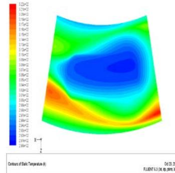
Figure 10: Temperature Field At 50rpm In Deficient State
