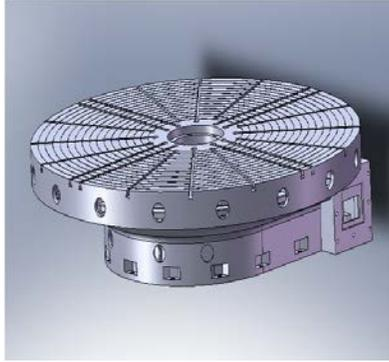
Figure 1: The Heavy Hydrostatic Bearing
