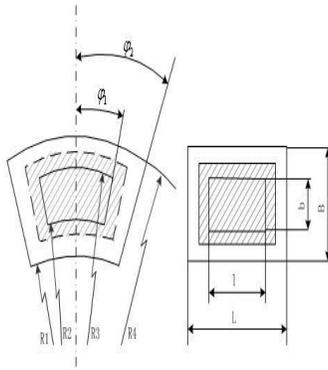
Figure 2: Sketch Map Of Separate Oil Pad With Sector Chamber
