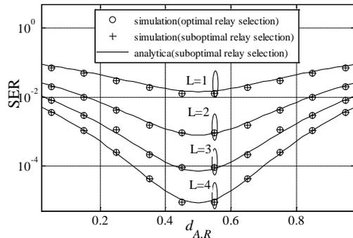
Fig. 8 SER Performance Against  $d_{A,R}$  When  $P_S = P_R = 5\text{dB}$
