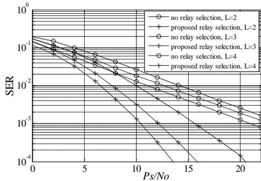
Fig. 3 SER Performance When  $P_R = P_S + 10\text{dB}$ .
