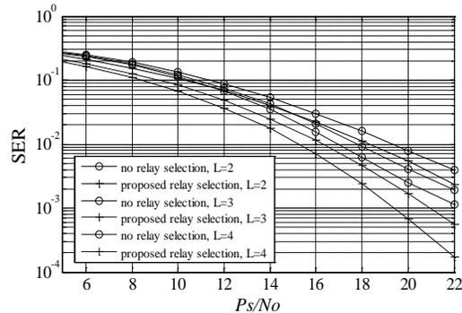
Fig. 4 SER Performance When  $P_R = P_S - 10\text{dB}$ .
