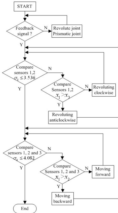
Figure 6. The Program Flowchart Of Automatic Centering
