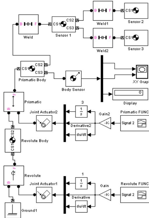
Figure 7. The Simmechanics Block Diagram Of Manipulator
