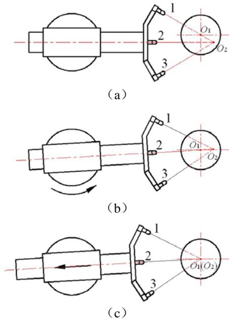
Figure 1. The Regulating Process Of Manipulator
