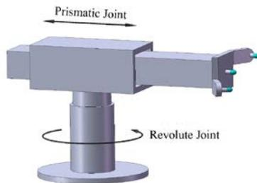
Figure 3. The Mechanism Diagram Of Manipulator
