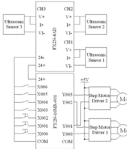
Figure 5. The Wiring Diagram Of PLC And A/D Converter
