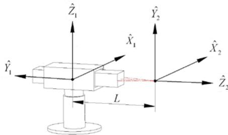
Figure 8. The Arrangement Of Manipulator's Coordinates
