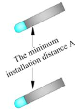
Figure 2. The Installation Distance Of Ultrasonic sensor
