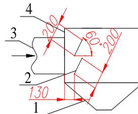
Figure 4. Guide Plates In The Cabinet (1. Ash Bunker, 2. Guide Plates, 3. Flue Gas Inlet, 4. Cabinet).
