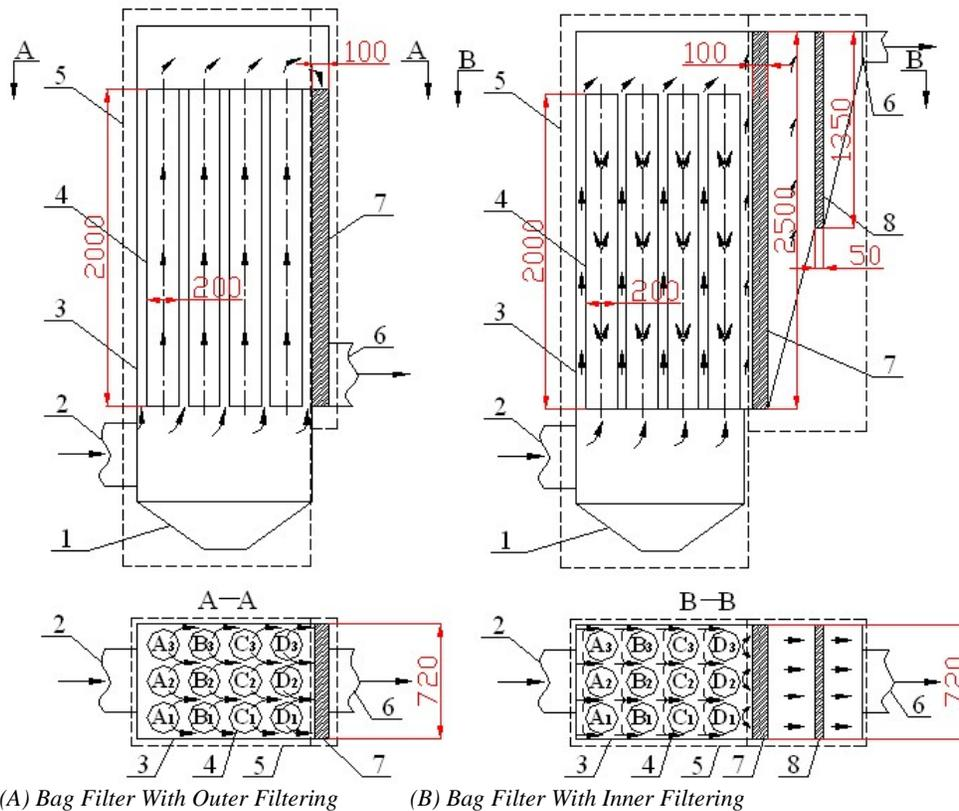
Figure 2. System Of Equipment Integrated PM2.5 And Mercury Removal.(1. Ash Bunker, 2. Flue Gas Inlet, 3. Cabinet, 4. Filter Bags, 5. Bag Filter, 6. Flue Gas Outlet, 7. AC Absorber I, 8. AC Absorber II).
