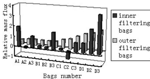
Figure 3. Relative gas mass flux in each bag without guide plates.
