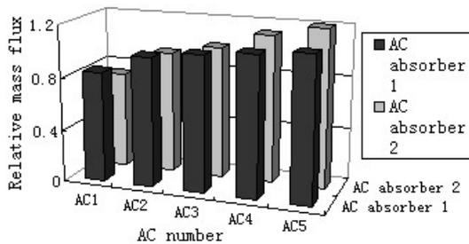
Figure 7. The Relative Gas Mass Flux For AC Absorbers With The Inner Filtering Bags.
