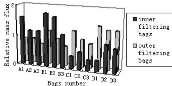
Figure 5. Relative Gas Mass Flux In Each Bag With Guide Plates.
