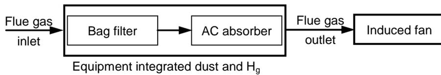
Figure 1. Flow chart of the equipment.
