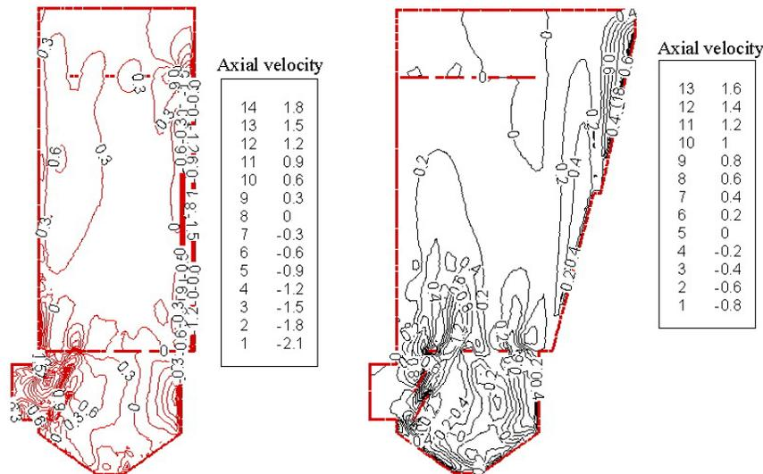
(A) Bag Filter With Outer Filtering. (B) Bag Filter With Inner Filtering.
