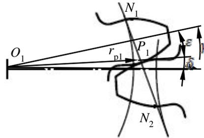
Figure 3: The Meshing Position When  $r_{p1} < r_p$
