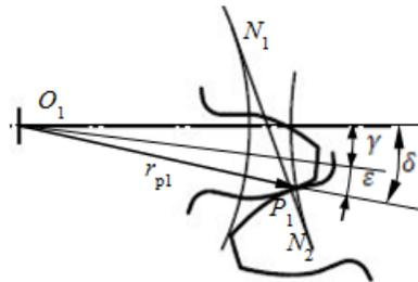
Figure 2: The Meshing Position When  $r_{p1} \geq r_p$
