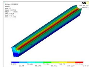
Figure 8: Equivalent Bending Stress Of Pinion
