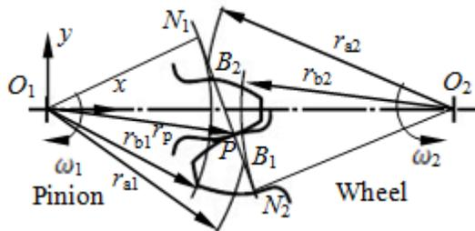
Figure 1: The Reference Meshing Position
