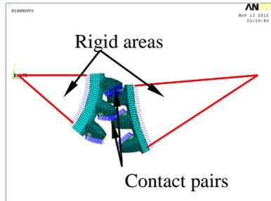
Figure 6: Contact Pairs And Rigid Areas
