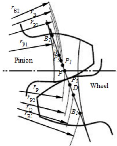
Figure 9: Positions Of The Meshing Points
