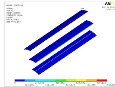
Figure 7: Contact Stress Of Pinion
