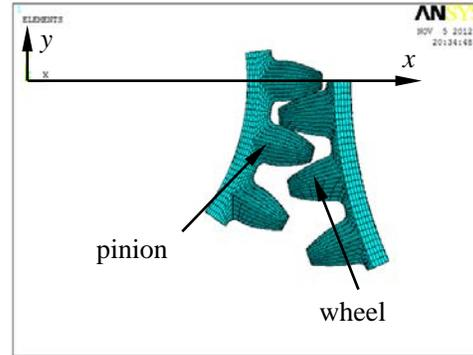
Figure 4: Gear Model At The Reference Position
