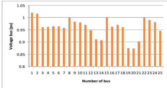
Fig.8. Voltage Profile Before Optimization Using TCSC
