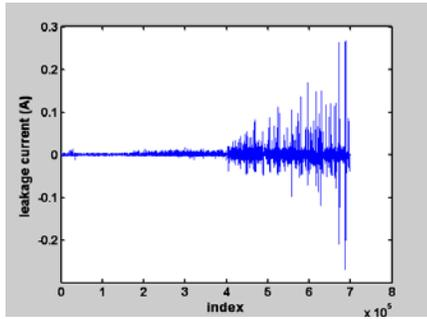
Figure 6: Leakage Current (ESDD=0.10)
