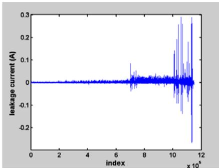
Figure 8: Leakage Current (ESDD=0.15)
