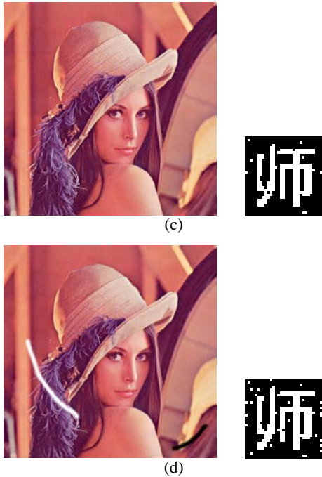
Figure 3: (a) Speckle noise attack(PSNR=19.39, BER=0.0471) (b) Image enhance attack(PSNR=19.01, BER=0.0209) (c) Image Sharpening attack(PSNR=38.75, BER=0.0166) (d) Random painting attack(PSNR=24.86, BER=0.0322)
