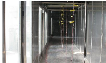
Figure 4: The Installation Of Thermocouples In The Corridor
