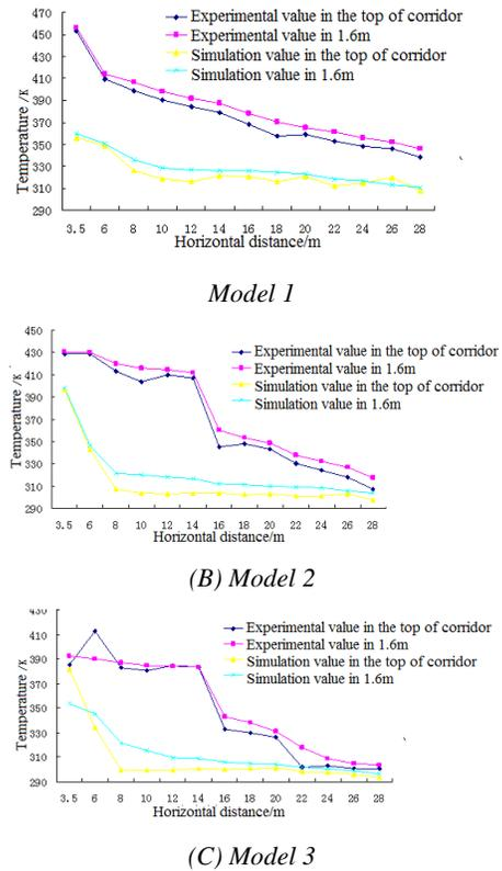
Figure 9: Temperature comparing of model 1-3 at 300s
