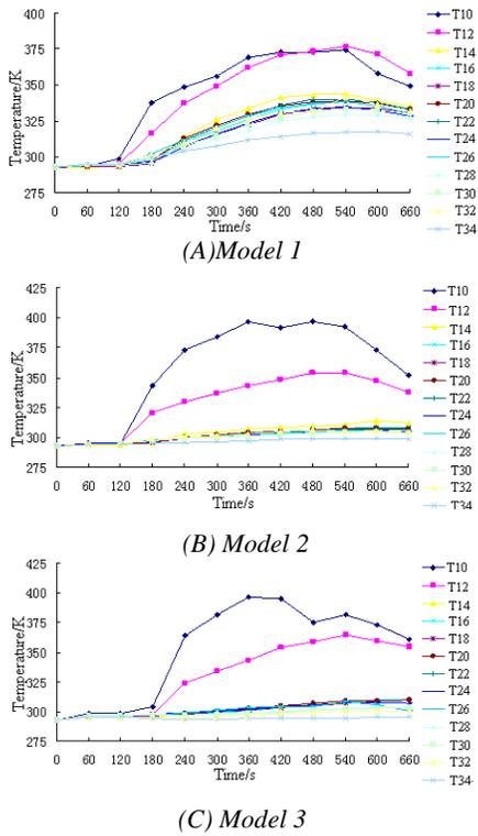
Figure 8: Temperature Distribution In The Gallery At The Height Of 1.6m
