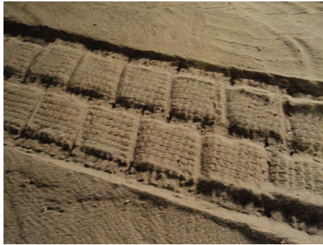
Figure 2: The Rutting In Lunar Soil Stimulant
