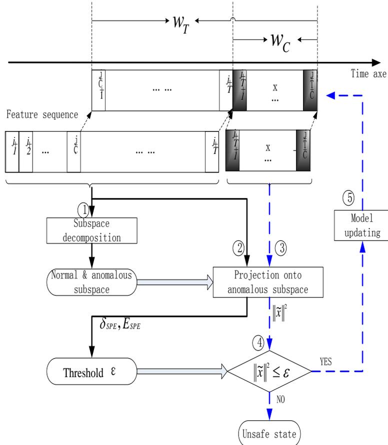
Figure 4: Unsafe State Detection Process
