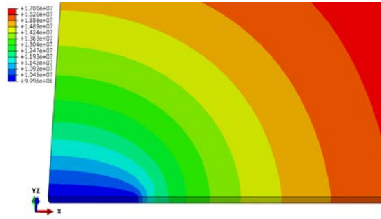
Figure 5: Pore Pressure Equivalence Contour Around The Hydraulic Fracture
