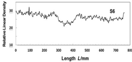
Figure 8: The Relative Linear Density Distribution Of Samples With Linear Defects
