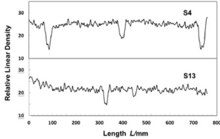
Figure 7: The Relative Linear Density Distribution Of Samples With Point-Like Defects
