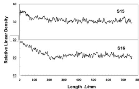
Figure 6: The Relative Linear Density Distribution Of Samples With Linear Density Of 25 G/M
