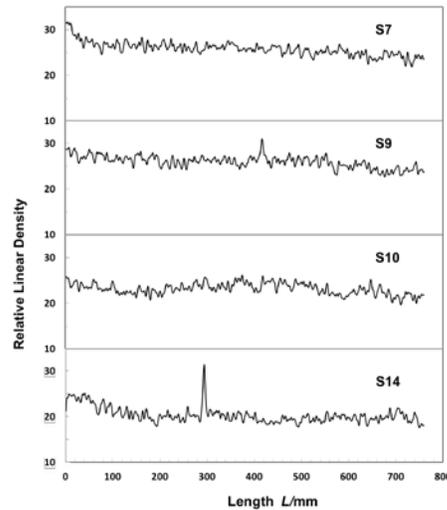
Figure 5: The Relative Linear Density Distribution Of Samples With Linear Density Of 22 G/M
