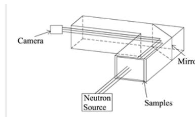
Figure 2: The Diagram Of Neutron Radiography Device
