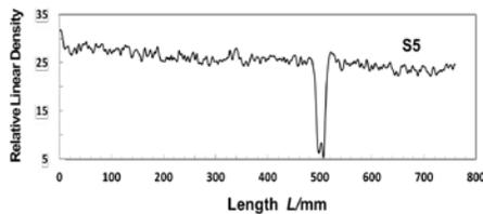
Figure 9: The Data Processing Result Of Samples With Planar Defects
