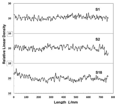
Figure 4: The Relative Linear Density Distribution Of Samples With Linear Density Of 6 G/M
