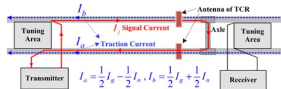
Figure 2: Signal And Traction Currents In Two Tracks
