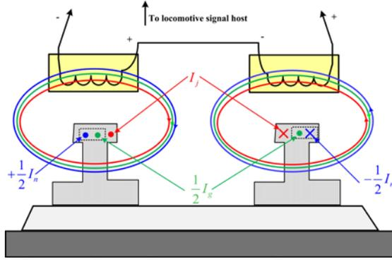
Figure 3: Ground-Train Information Transmission And ITC Formation Mechanism
