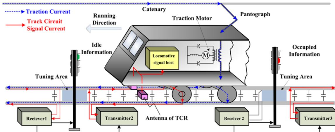
Figure 1: Diagram Of The Operating Principal Of Track Circuits And Traction Currents
