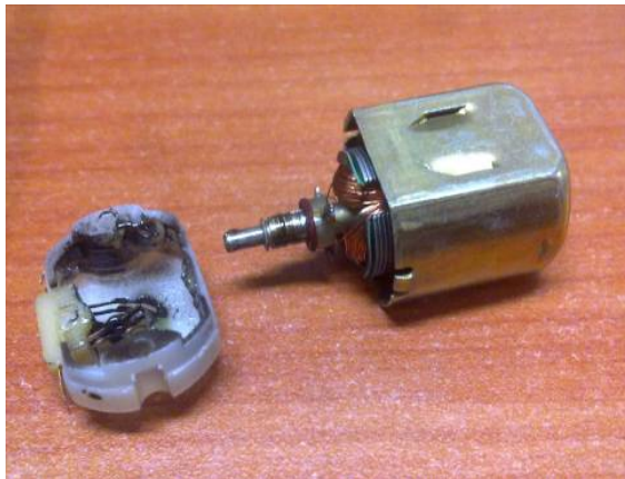
Figure 2 Dc Motor Failure Mechanism
