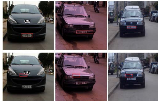
Figure 3: Some Examples Of Vehicle License Plate Detection Process Outputs. (Top) The Results Of The New Proposed Approach, And (Down) Those Of The Method Given By [15].
