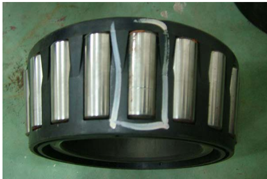
Figure 3: Wheelset Bearing With Rolling Element Electric Erosion Fault
