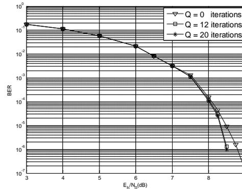
Figure 4: Serial concatenated coded  $M$ -ary modulation system BER performance with iteration schemes in AWGN channel, and the spectral efficiency is 1.5b/s/Hz. (Parameters: information frame length: 1536; convolution code generator polynomial is (5, 7)<sub>8</sub>; 8-CPM ( $h=1/2$ ))
