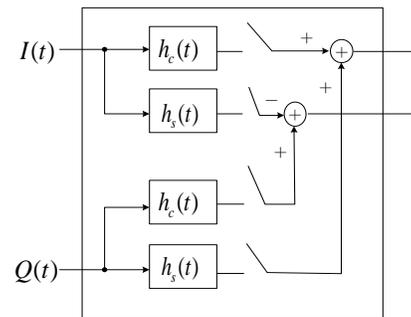
Figure 2b: The Architecture Of Matched Filter
