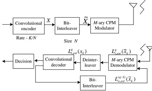
Figure 1: Block Of Serially Concatenated Coded M-Ary CPM With Bit-Interleaver: Transmitter And Receiver
