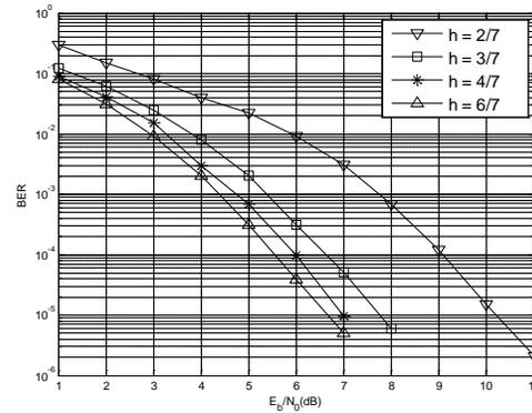
Figure 3: 4-Ary CPM System ( $N = 1000$ ) BER Performance With Different Modulation Index In AWGN Channel
