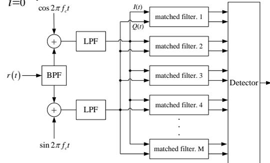
Figure 2a: The Architecture Of CPM Optimal Receiver
