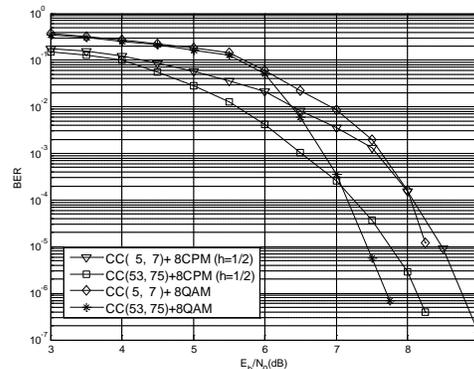
Figure 5: Serial concatenated coded  $M$ -ary modulation system BER performance with different modulation schemes in AWGN channel, and the spectral efficiency is 1.5b/s/Hz. (Parameters: information frame length: 1536; convolutional code generator polynomial are (5, 7)<sub>8</sub> and (53, 75)<sub>8</sub>; 8-ary CPM ( $h=1/2$ )).
